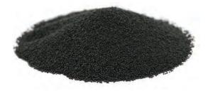
PS Ball is an abrasive that is produced by super- cooling molten steel slag. It is suitable for a wide range of applications, and its most common usage is as an abrasive for the surface preparation of steel prior to the application of paint coatings.
